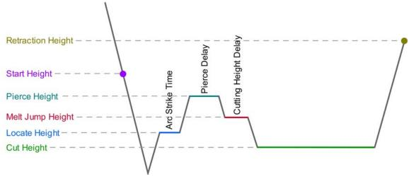
Start Height - manually entered value on the 'Machine' menu. Pressing K2 causes the torch to move downwards at it's fastest speed to the 'Start Height', slow to IHS speed, and then continue moving downward until it senses the material. It then raises up to 'Locate Height' (this option will only appear if '485 THC' has been selected on the 'Machine' tab, p 28).
