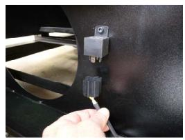
The exhaust fan has two cables extending out of it - a three position power cord, and a two wire cable. Again, make sure the power cable is unplugged before continuing. Locate the two wire cable and unwrap the electrical tape, exposing the two female connectors. Pass the connectors and cable through the small hole in the electrical panel:
