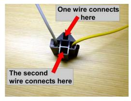
Finish the installation by plugging the black electrical block back into the relay. Due to the design of the electrical block, there is only one correct orientation of the terminals.
