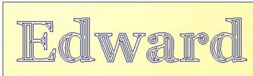
Fill engraving with Offset pattern
