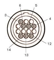
Wires 3 and 4 are inputs, and control the start circuit inside the plasma cutter. A switched signal from the plasma controller turns the plasma cutter on or off.
